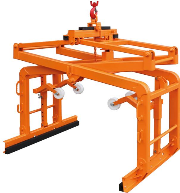
Specifically designed and developed for the UK market to lift palletized brickloads (Note: bricks must be securely bound). Suitable for handling all types of concrete products such as slabs, steel-strapped bricks, blocks kerb stones and paving blocks. palletized bound loads. Lined with hard rubber pads to minimise damage to load.
